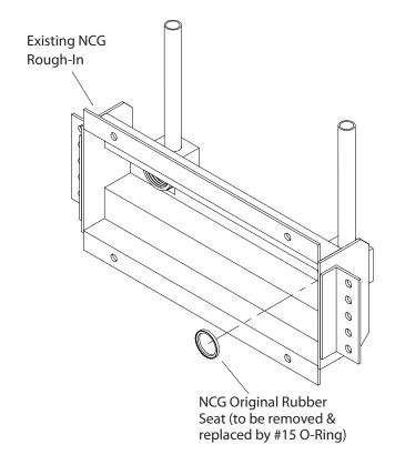
**Step 2:** Thread the Amico Retro-Fit rough-in assembly to the existing NCG rough-in.
