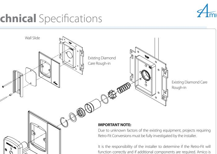
NOTE: Suction inlets are not supplied with a secondary check valve. A pressure plug is provided for testing purposes, rated at 150 psi [1,034 kPa].
