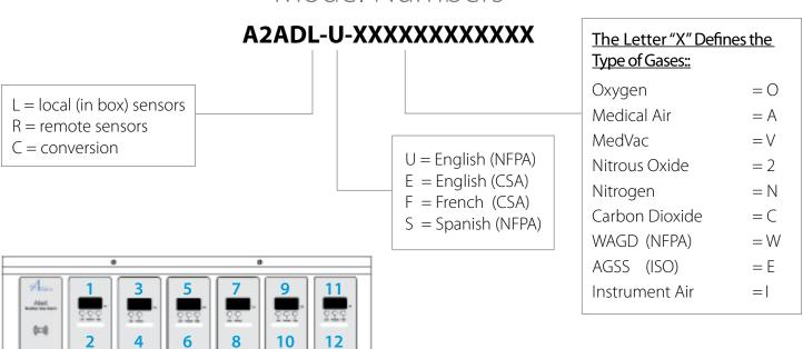
"X" indicates the order of gases, as shown above. **example:** OAV (position 1 OXY, position 2 AIR, position 3 VAC)
