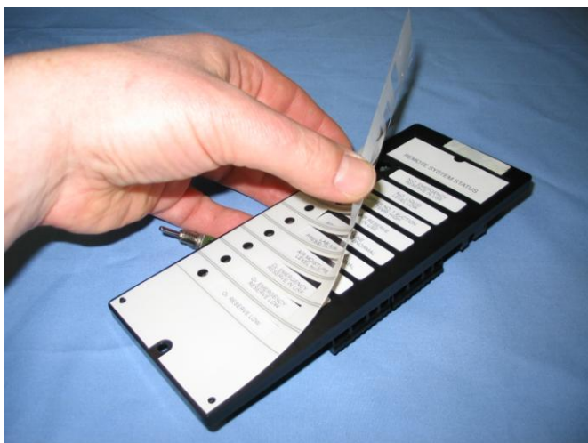
Figure 19 – Labeling 10 Switch Signal Module
