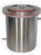
DryIce/Liquid Nitrogen Cold Trap is an effective foreline cold trap for vacuum manifolds or Schlenk Lines. The trap has a large 3 quart (2.8 liters) center well for the dry ice/isopropyl alcohol slurry or liquid nitrogen; traps up to 1.5 liter condensate. With dry ice cold temperature may be maintained for up to 12 hours depending upon the vapor load. With liquid nitrogen cold temperature can be maintained for up to 2 hours depending upon the vapor load.
