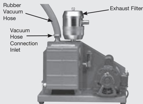
**Exhaust Filter** - Connects to pump's outlet. Filters oil mist from the pump's exhaust to keep your working area clean and air quality healthful. A second option is an exhaust line to a vapor hood or other outside exhaust vent. This requires an adapter and air tight connections (see p. 40).
