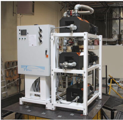
Unit Under Test UUT14: Triplex Stack Mounted Contact-less Claw Vacuum System
